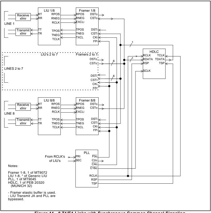
Figure 11 - 8 T1/E1 Links with Synchronous Common Channel Signaling
