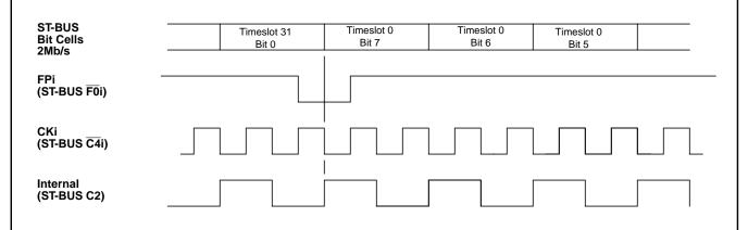
Figure 25 - ST-BUS 2.048Mb/s Functional Timing Diagram
