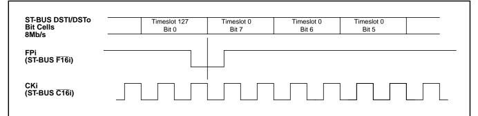
Figure 27 - ST-BUS 8.192Mb/s Functional Timing Diagram for DSTi/DSTo
