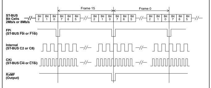
Figure 56 - E1 Receive Multiframe (CRC-4 or CAS) Functional Timing with Tx8KEN Set to 0
