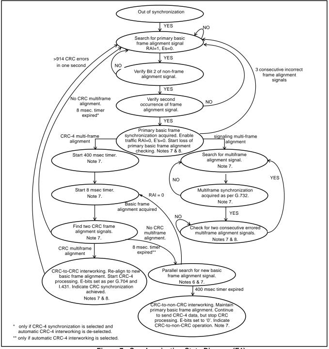
Figure 7 - Synchronization State Diagram (E1)
