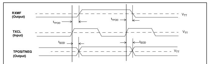
Figure 38 - T1 Receive Multiframe Timing with TX8KEn Set to 1
