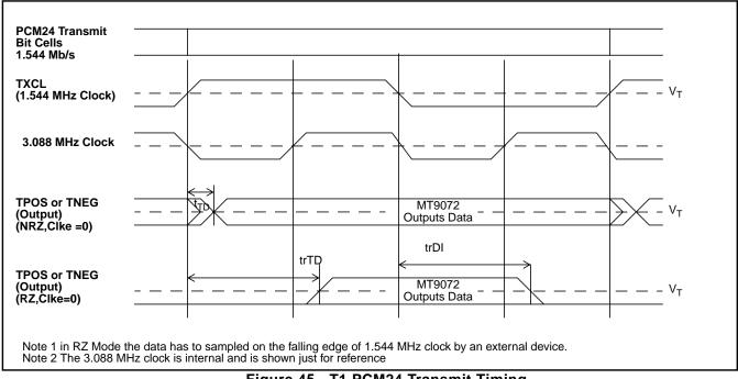
Figure 45 - T1 PCM24 Transmit Timing
