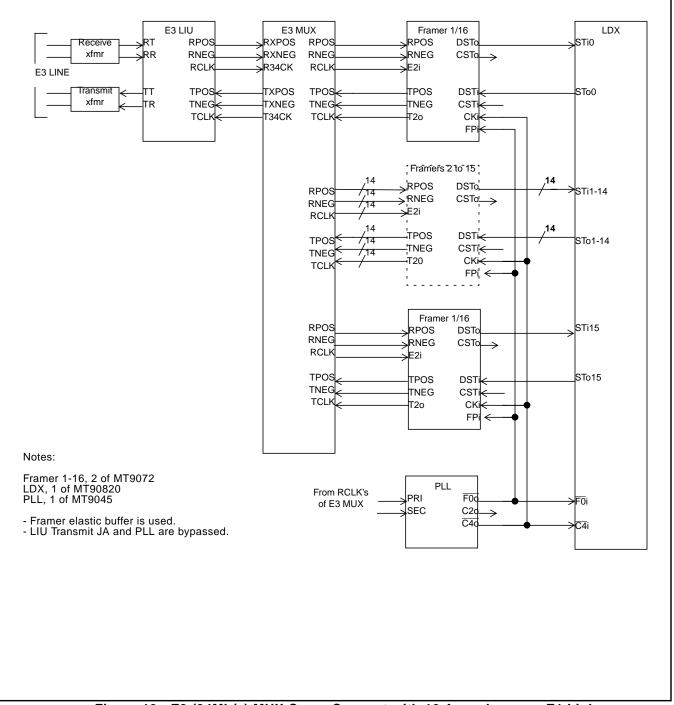
Figure 19 - E3 (34Mb/s) MUX Cross Connect with 16 Asynchronous E1 Links
