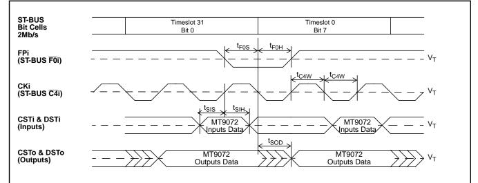
Figure 24 - ST-BUS 2.048Mb/s Timing
