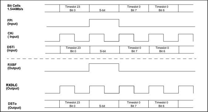
Figure 33 - T1 IMA Functional Timing Diagram
