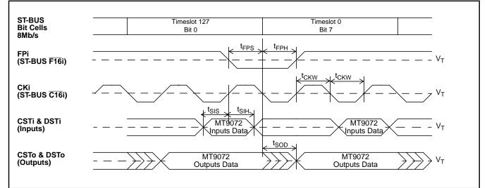
Figure 26 - ST-BUS 8.192Mb/s Timing
