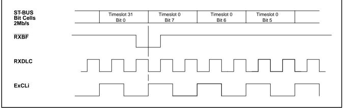
Figure 52 - E1 Receive IMA Functional Timing
