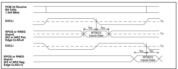
Figure 47 - T1 PCM24 Receive Timing
