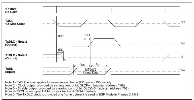
Figure 40 - Transmit Data Link Pin Timing
