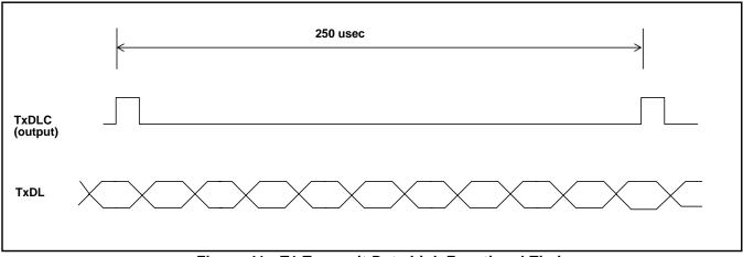
Figure 41 - T1 Transmit Data Link Functional Timing
