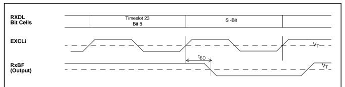
Figure 44 - T1 Receive Basic Frame Pulse Pin Timing
