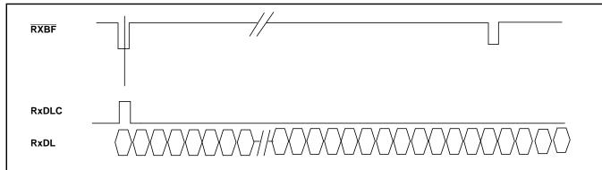
Figure 43 - T1 Receive Data Link Functional Timing
