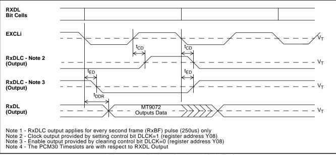
Figure 62 - E1 Receive Data Link Timing
