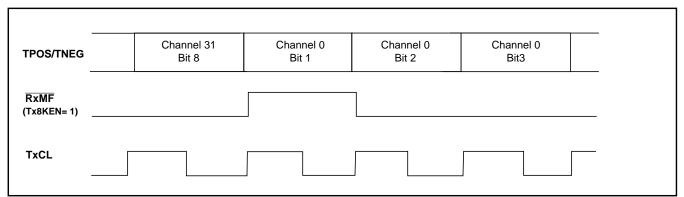
Figure 58 - E1 Receive Multiframe Timing with TX8KEn Set to 1
