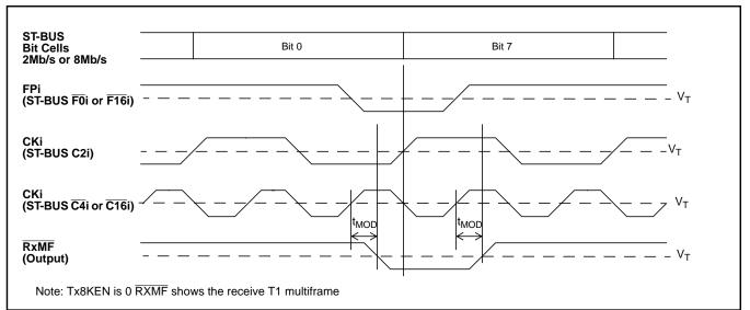
Figure 36 - T1 Receive Multiframe Timing with Tx8KEN Set to 0
