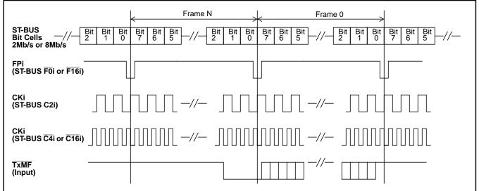
Figure 35 - T1 Transmit Multiframe Functional Timing
