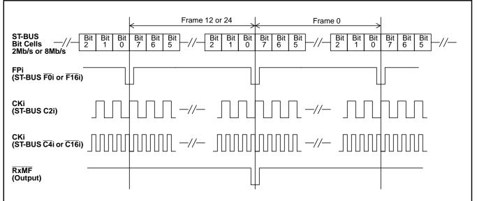
Figure 37 - Receive Multiframe Functional Timing with Tx8KEN Set to 0
