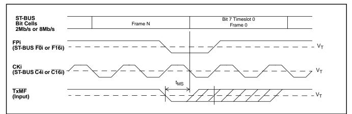
Figure 53 - E1 Transmit Multiframe (CRC-4 or CAS) Timing
