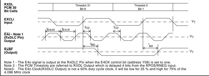
Figure 61 - E1 Receive Basic Frame and E40 Timing
