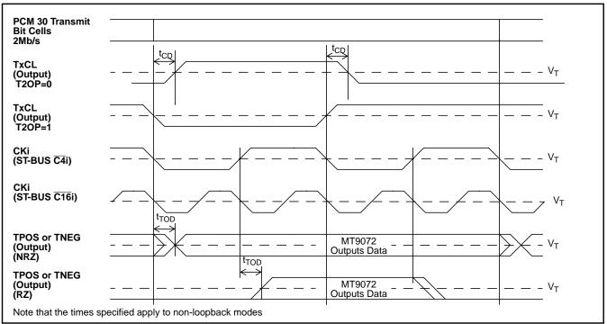
Figure 64 - E1 PCM30 Transmit Timing
