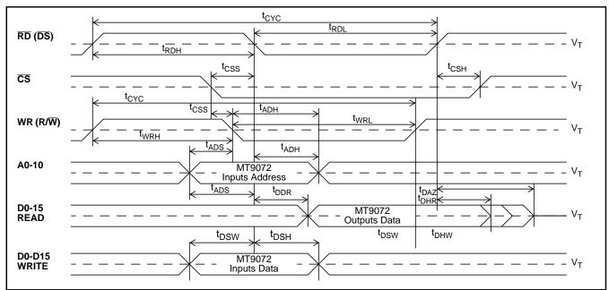
Figure 23 - Intel Microprocessor Timing
