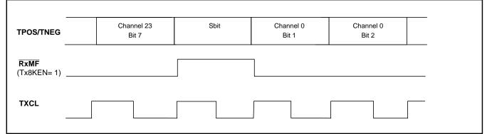
Figure 39 - T1 Receive Multiframe Timing Functional Timing Diagram with TX8KEn Set to 1
