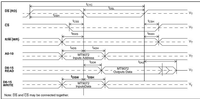
Figure 22 - Motorola Microprocessor Timing
