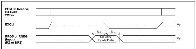
Figure 66 - E1 PCM30 Receive Timing
