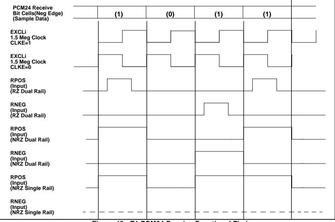
Figure 48 - T1 PCM24 Receive Functional Timing
