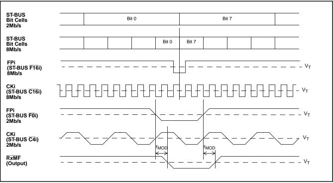
Figure 55 - E1 Receive Multiframe (CRC-4 or CAS) Timing with Tx8KEN Set to 0
