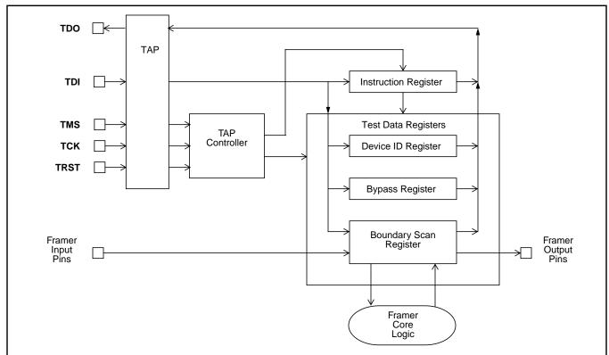
Figure 10 - Boundary Scan Test Circuit Block Diagram
