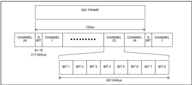
Figure 4 - PCM24 Link Frame Format (T1)
