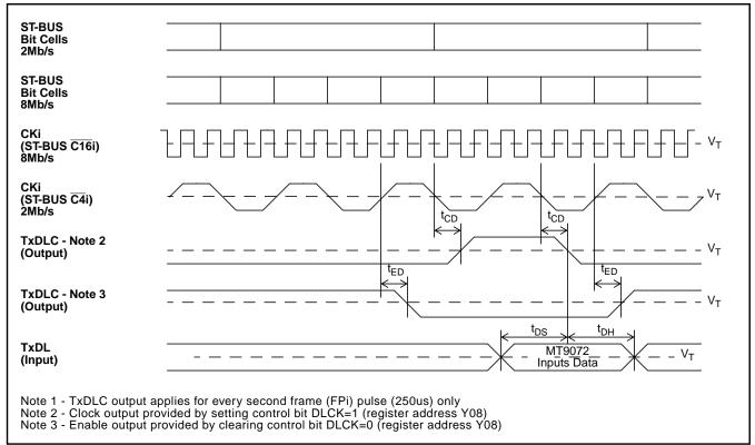
Figure 59 - E1 Transmit Data Link Pin Timing
