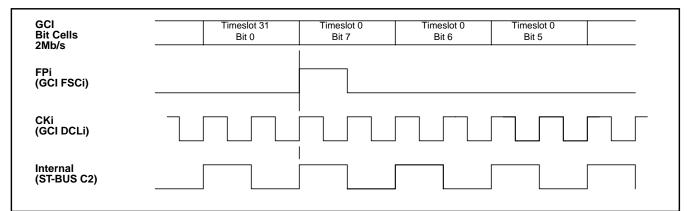
Figure 31 - GCI 2.048Mb/s Functional Timing Diagram
