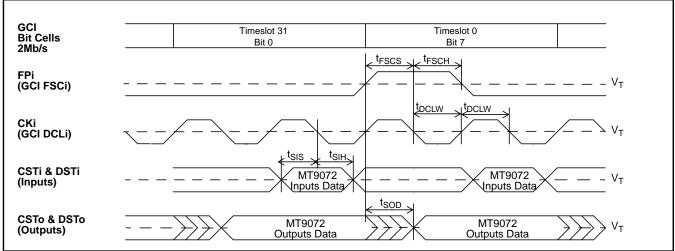
Figure 30 - GCI 2.048 Mb/s Timing Diagram
