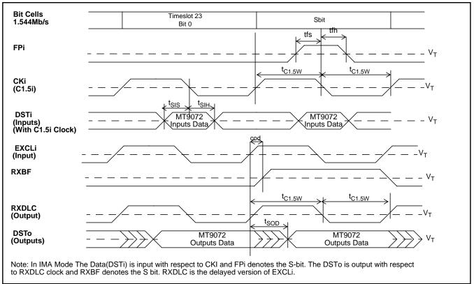
Figure 32 - T1 IMA Mode Timing Diagram
